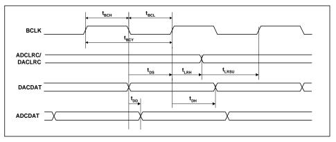
Figure 3 Digital Audio Data Timing - Slave Mode
