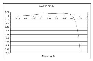
Figure 43 DAC Digital Filter Ripple (Sloping Stopband Mode)
