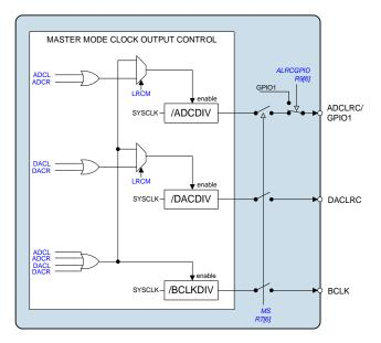
Figure 33 Master Mode Clock Output Control
