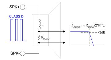
Figure 50 Speaker Equivalent Circuit
