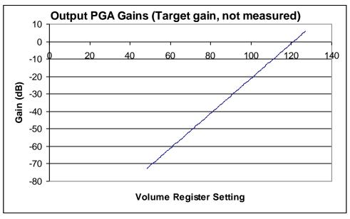
Figure 1 Output PGA Gains (LOUT1VOL, ROUT1VOL, SPKLVOL, SPKRVOL)
