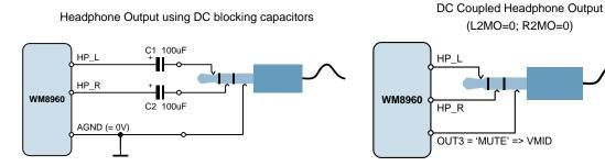
Figure 15 Recommended Headphone Output Configurations
