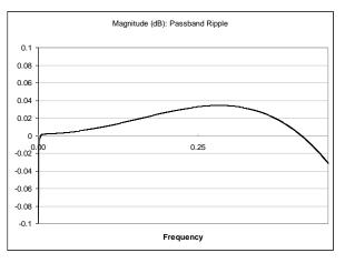
Figure 38 ADC Digital Filter Frequency Response
