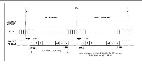
Figure 28 I<sup>2</sup>S Justified Audio Interface (assuming n-bit word length)
