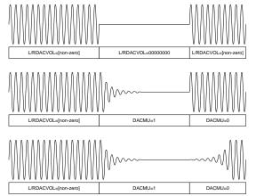
DAC muting and un-muting using volume control bits LDACVOL and RDACVOL.
