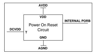
Figure 5 Internal Power on Reset Circuit Schematic
