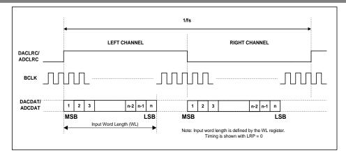
Figure 26 Left Justified Audio Interface (assuming n-bit word length)
