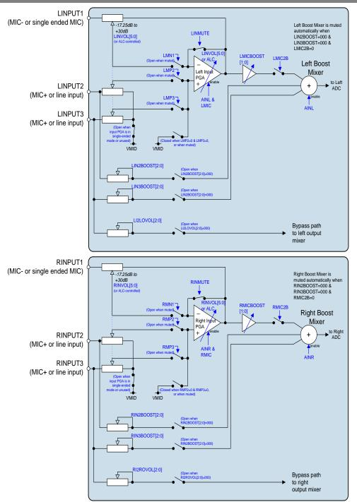
Figure 8 Microphone Input PGA Circuit
