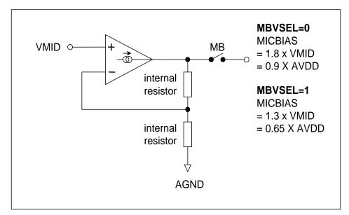
Figure 9 Microphone Bias Schematic
