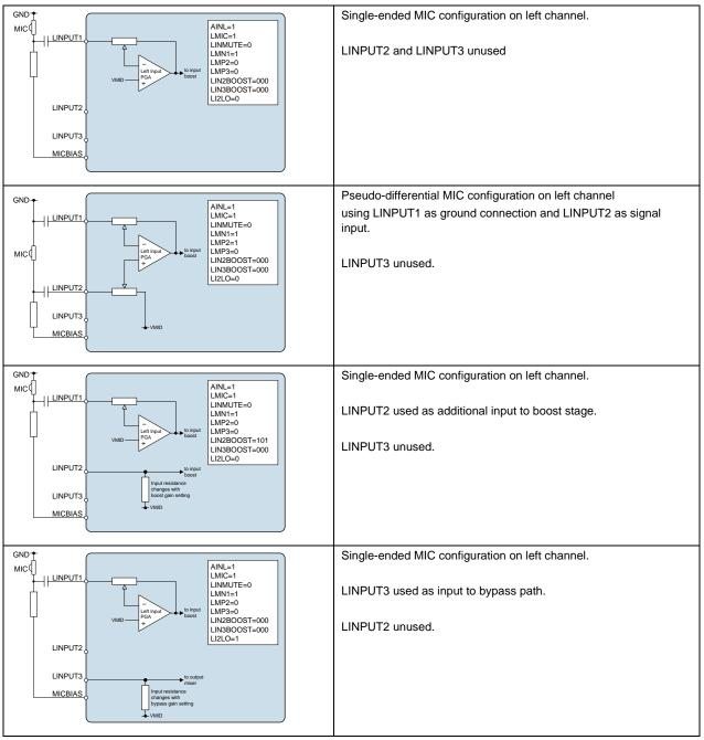
Figure 10 Example Microphone Input Configurations (See also "Recommended External Components")
