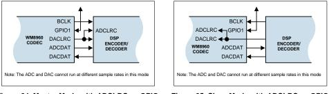
Figure 24 Master Mode with ADCLRC as GPIO
