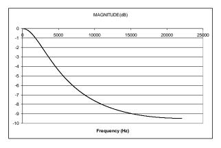
Figure 46 De-Emphasis Digital Filter Response (44.1kHz)
